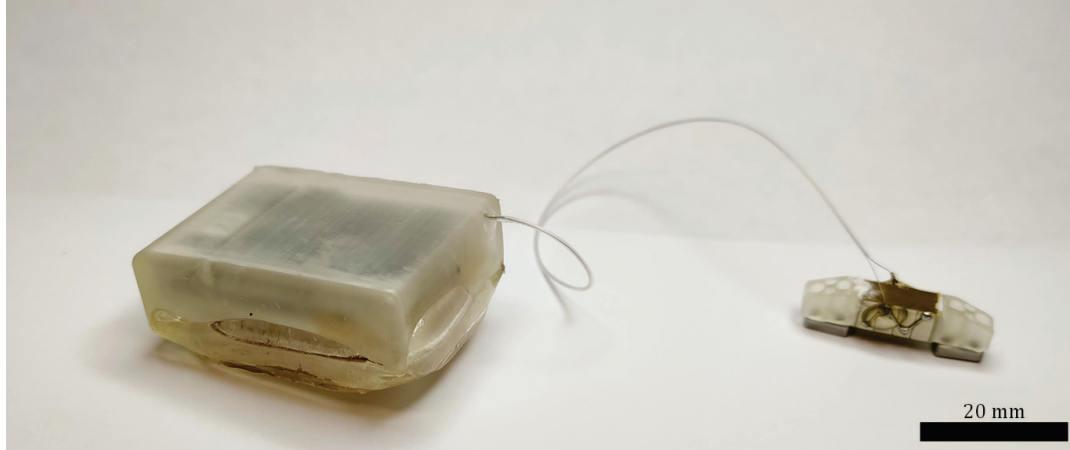
Figure 1.5 Complete implantable device consisting of a telemetry unit (left) wired to the fixation plate (right). The telemetry unit has dimensions 42.8 x 31.4 x 15.0 mm. The fixation plate without riser plates has dimensions 5 x 5 x 25.6 mm.
