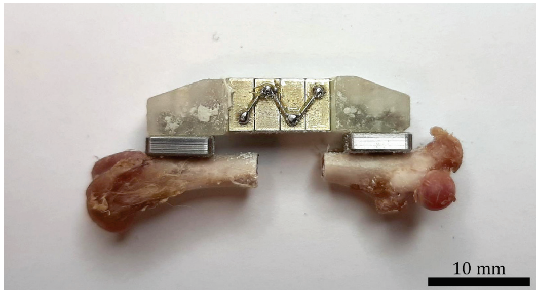
Figure 3.27 Fixator attached to explanted rat femur via screws. The defect size is 6 mm.
